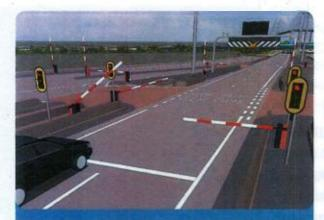
Barriers will be used in conjunction with traffic signals to stop vehicles and enforce crossing restrictions when required.
