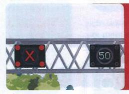
Signs on gantries over the carriageway will display variable speed limits to keep traffic flowing safely, dependant on the road conditions at the time.
